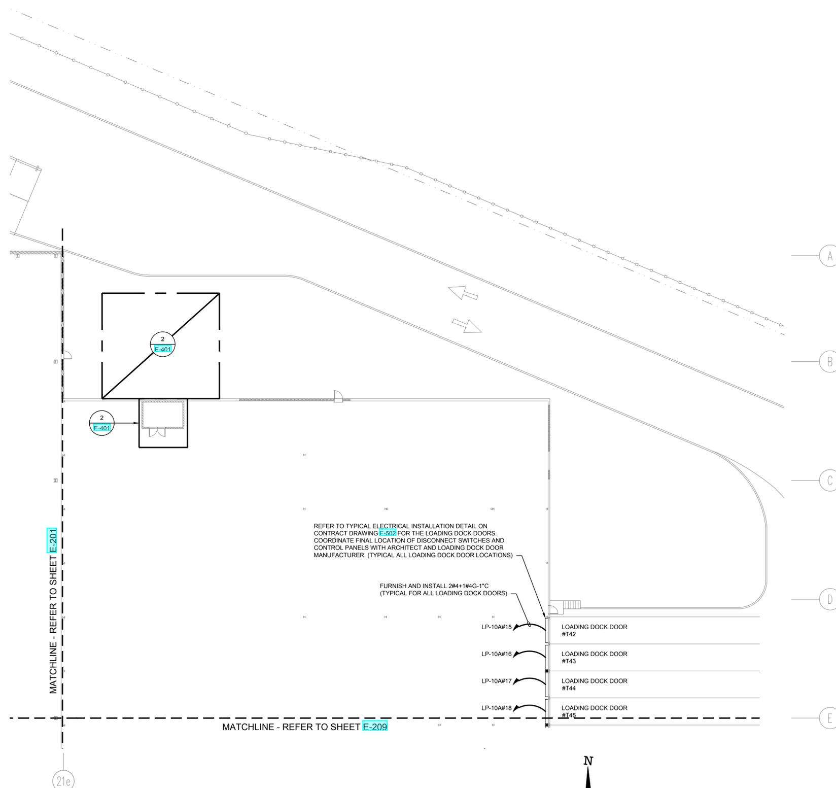
REFER TO TYPICAL ELECTRICAL INSTALLATION DETAIL ON CONTRACT DRAWING E-502 FOR THE LOADING DOCK DOORS. COORDINATE FINAL LOCATION OF DISCONNECT SWITCHES AND CONTROL PANELS WITH ARCHITECT AND LOADING DOCK DOOR MANUFACTURER. (TYPICAL ALL LOADING DOCK DOOR LOCATIONS)
