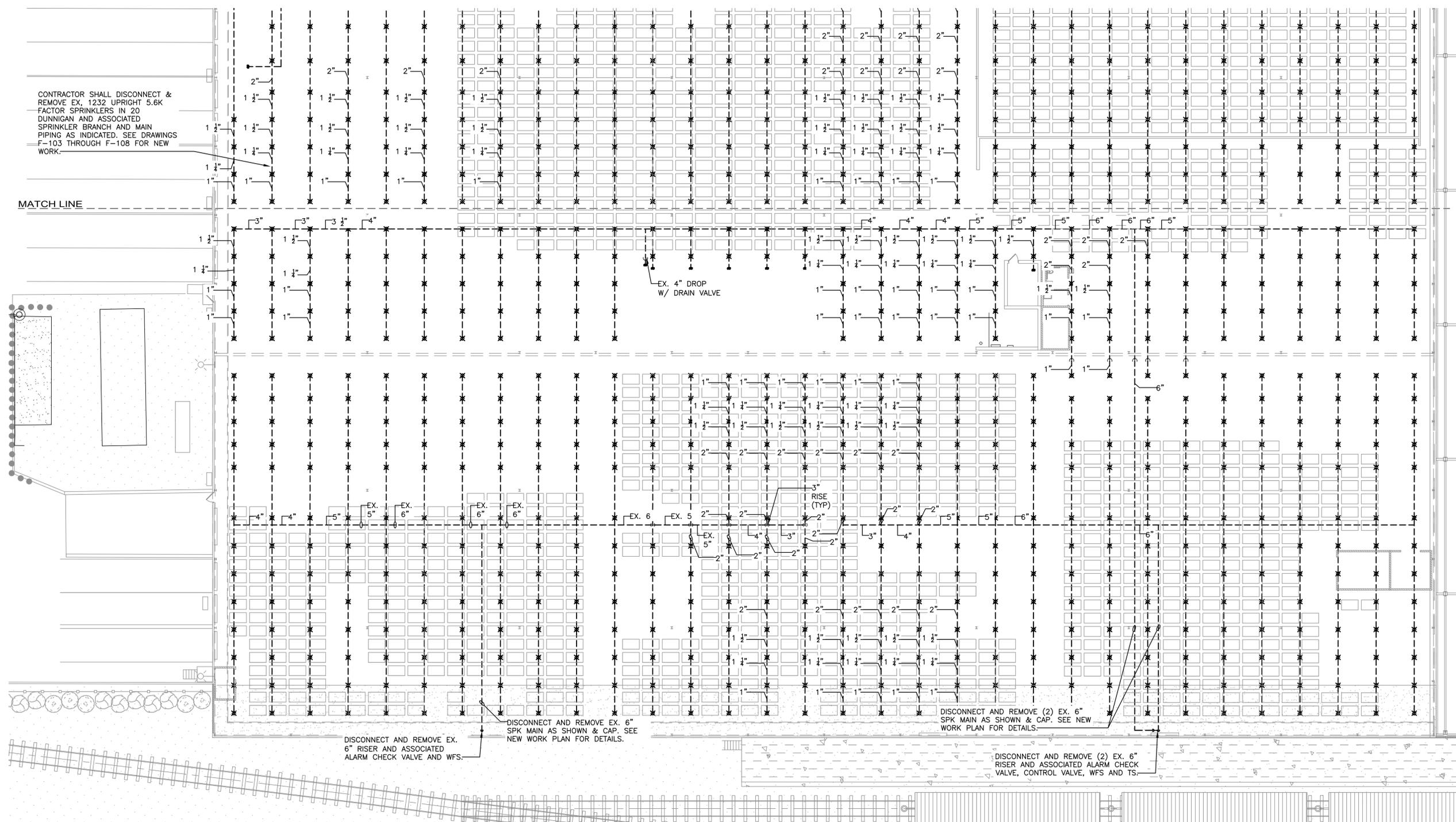
CONTRACTOR SHALL DISCONNECT & REMOVE EX. 1232 UPRIGHT 5.6K FACTOR SPRINKLERS IN 20 DUNNIGAN AND ASSOCIATED SPRINKLER BRANCH AND MAIN PIPING AS INDICATED. SEE DRAWINGS F-103 THROUGH F-108 FOR NEW WORK.
