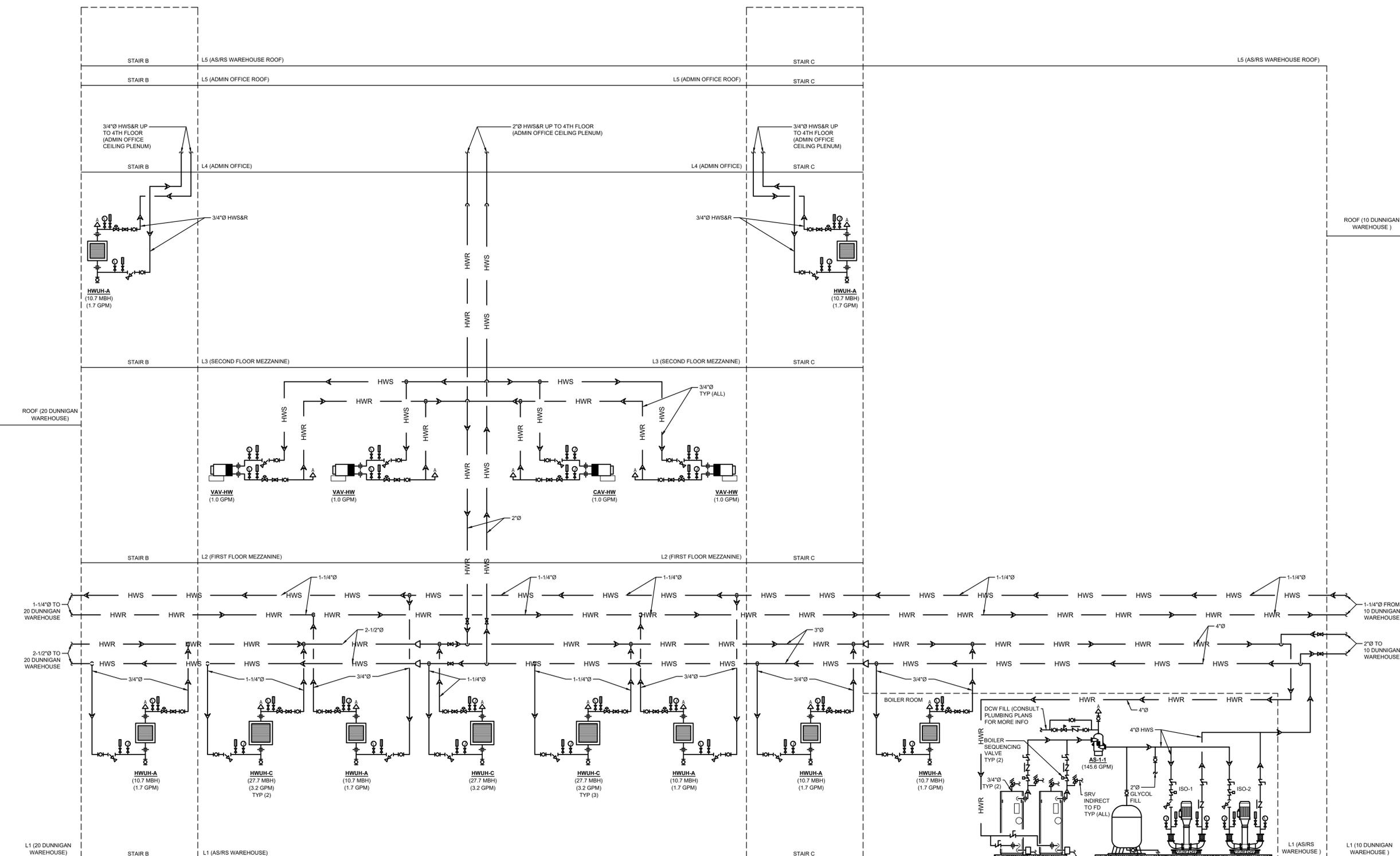
**1 MECHANICAL HOT WATER FLOW DIAGRAM-AS/RS WAREHOUSE**
