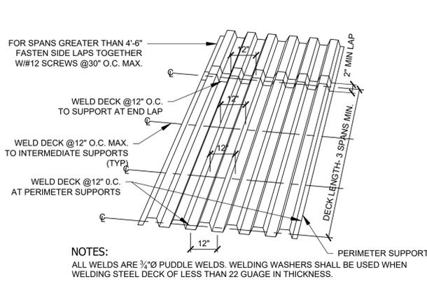
1 TYP. SLAB DECK WELDING
