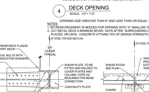
5 TYPICAL DECK SUPPORT AT BEAM MOMENT CONNECTION TO COLUMN WEB
