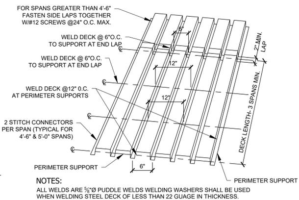
2 TYP. SLAB ROOF WELDING
