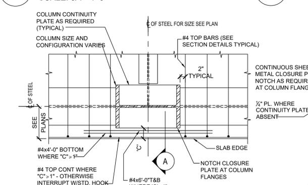
8 TYPICAL SLAB REINFORCING AT EXTERIOR COLUMNS
