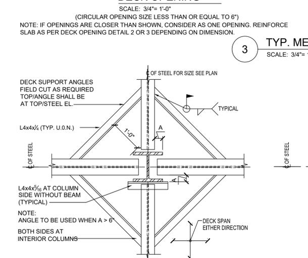
3 TYPICAL DECK SUPPORT AT INTERIOR OR EXTERIOR COLUMNS
