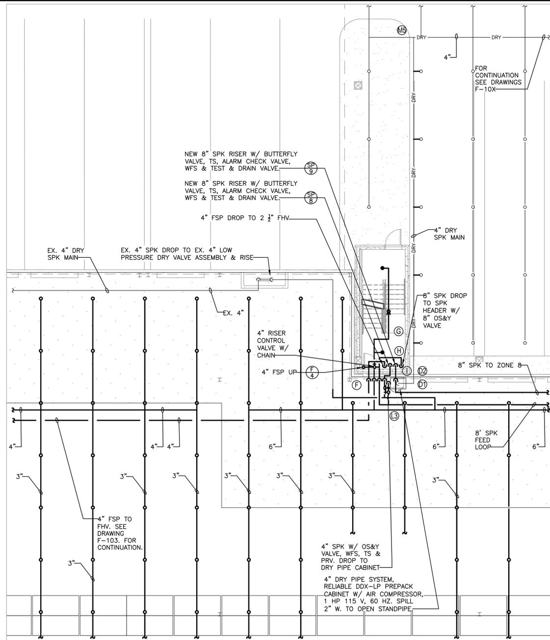
1 FIRE PROTECTION STAIR A PART PLAN
