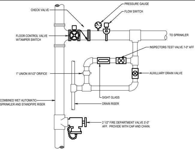
**COMBINED WET AUTOMATIC SPRINKLER AND STANDPIPE RISER FLOOR CONTROL VALVE ASSEMBLY**
