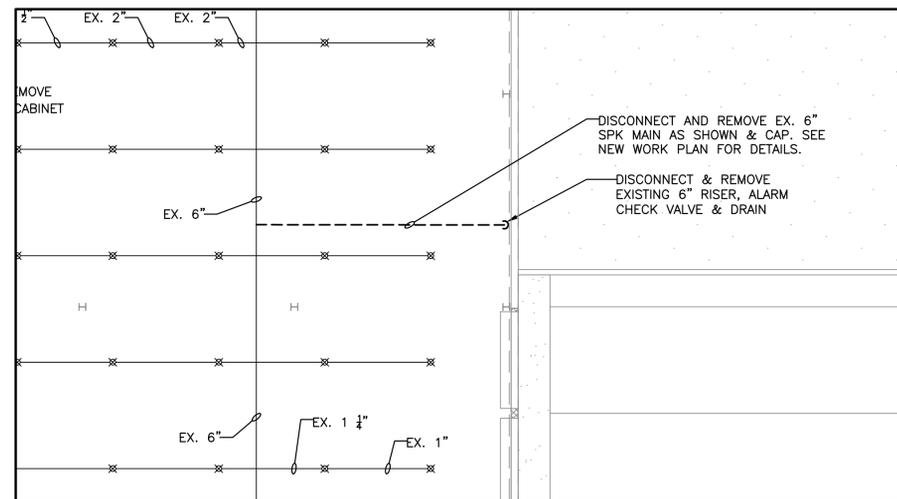
**1st FLOOR DEMOLITION PART PLAN**
