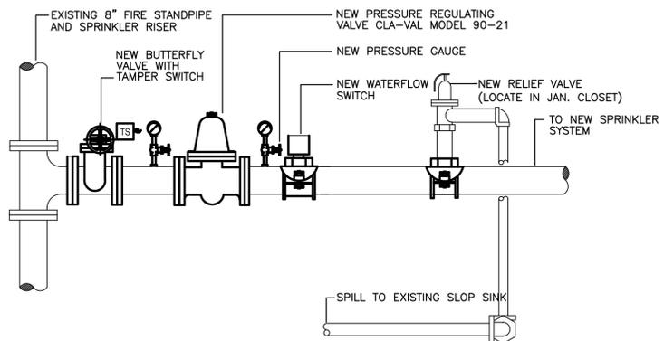
**NEW FLOOR CONTROL VALVE ASSEMBLY WITH P.R.V.**
