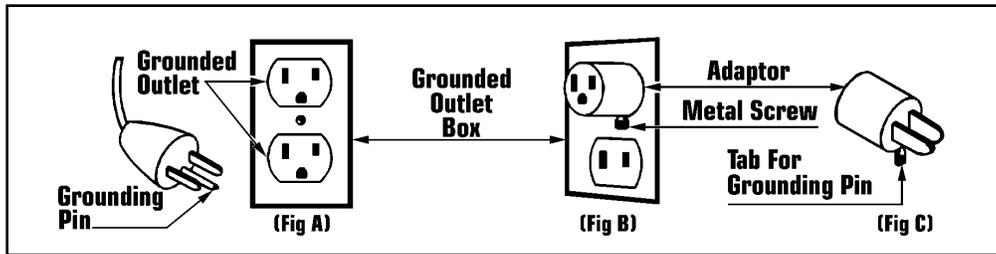
This electric equipment is for use on a nominal 120 volt circuit, and has a grounded plug that looks like the plug illustrated in (Fig A). A temporary adaptor that looks like the adaptor illustrated in (Fig B & C) may be used to connect this plug to a 2-pole receptacle as shown in (Fig B) if a properly grounded outlet is not available.
