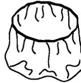
The 2-ply intermediate filter should be replaced with every fifth change of paper bag and whenever there is damage or a visible collection of debris on the outside of the filter.
