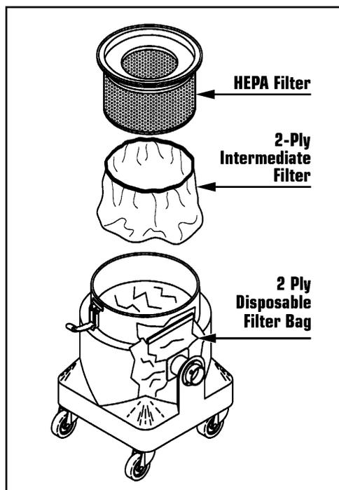
The 2-ply intermediate filter is a very fine non-woven filter that extends the life of the expensive High-Efficiency Particulate Air (HEPA) filter.
