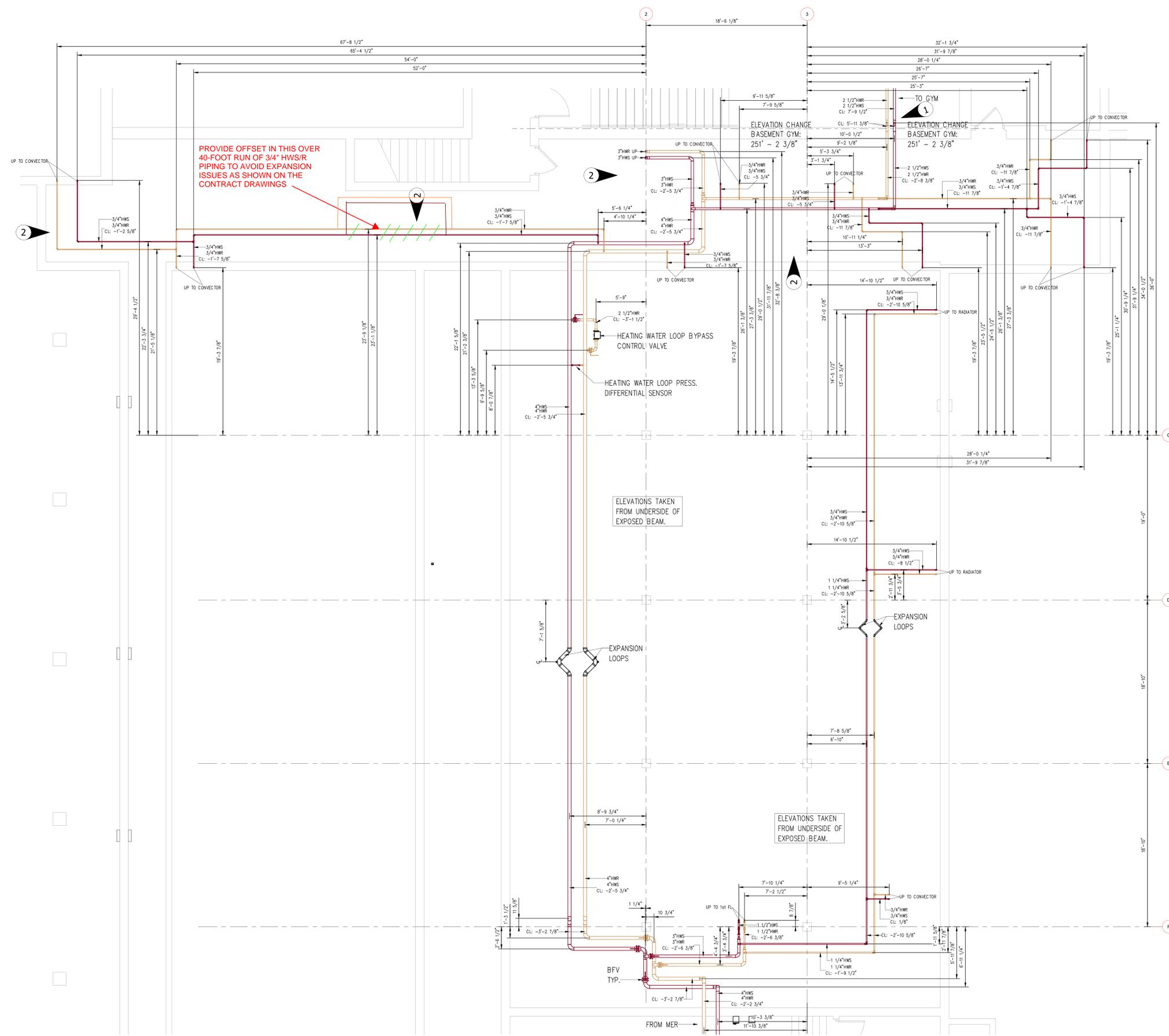
PROVIDE OFFSET IN THIS OVER 40-FOOT RUN OF 3/4\"/>
