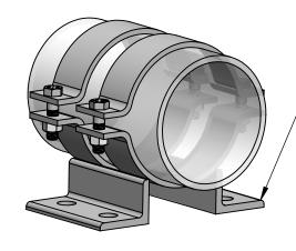
FEET CAN BE BOLTED OR WELDED TO STRUCTURE
