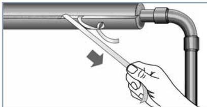
Peel the protective release strips from the adhesive surface in 8" and 12" increments *after* insulation is snapped over pipe. The protective release strips can be removed by gently pulling at an angle. Apply firm and even pressure along the entire longitudinal seam for proper seal.
