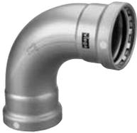
MegaPress FKM is a carbon steel, cold press system designed for use in chilled water, hydronic heating, compressed air, and fire sprinkler applications. MegaPress FKM fittings in sizes from ½" to 4" are offered
