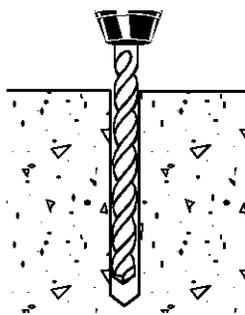
Insert anchor into the hole, threaded cone end first until the outer sleeve is flush with the surface of the base material.
