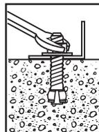
4. Expand anchor by tightening nut 3-5 turns past the hand tight position, or to the specified torque requirement.
