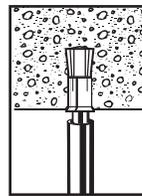
4. Expand anchor with setting tool provided (see chart). Anchor is properly expanded when shoulder of setting tool is flush with top of anchor.
