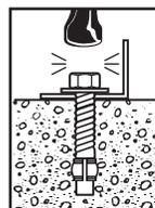
3. Assemble washer and nut, leaving nut flush with end of anchor to protect threads. Drive anchor through material to be fastened until washer is flush to surface of material.
