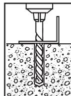
1. Select a carbide drill bit with a diameter equal to the anchor diameter. Drill hole to any depth exceeding the desired embedment. See chart for minimum recommended embedment.
