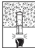
3. Drive anchor flush with surface of concrete.
