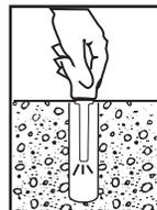
2. Clean hole or continue drilling additional depth to accommodate drill fines.
