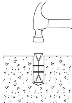
Position fixture, then insert screw or bolt and tighten. For maximum expansion, the upper cone should protrude slightly before setting. The bolt must engage a minimum of 2/3 of the anchor threads.
