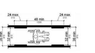
FIG. 403.5.1 CLEAR WIDTH OF AN ACCESSIBLE ROUTE
