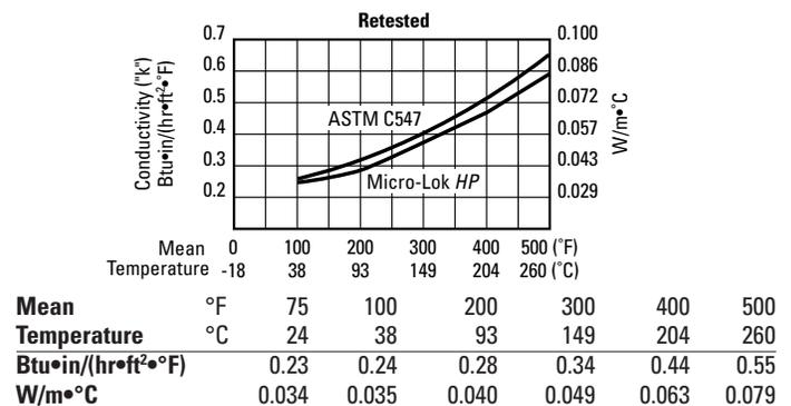
\* Apparent thermal conductivity values are determined by applying procedures dictated per ASTM C1045 on test data obtained using ASTM Test Method C335. All values are based on nominal manufacturing and testing parameters, are subject to normal variation, and are not guaranteed for specification purposes or otherwise.
