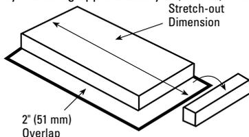
Before applying duct wrap, sheet metal duct shall be clean, dry and tightly sealed at all joints and seams.
