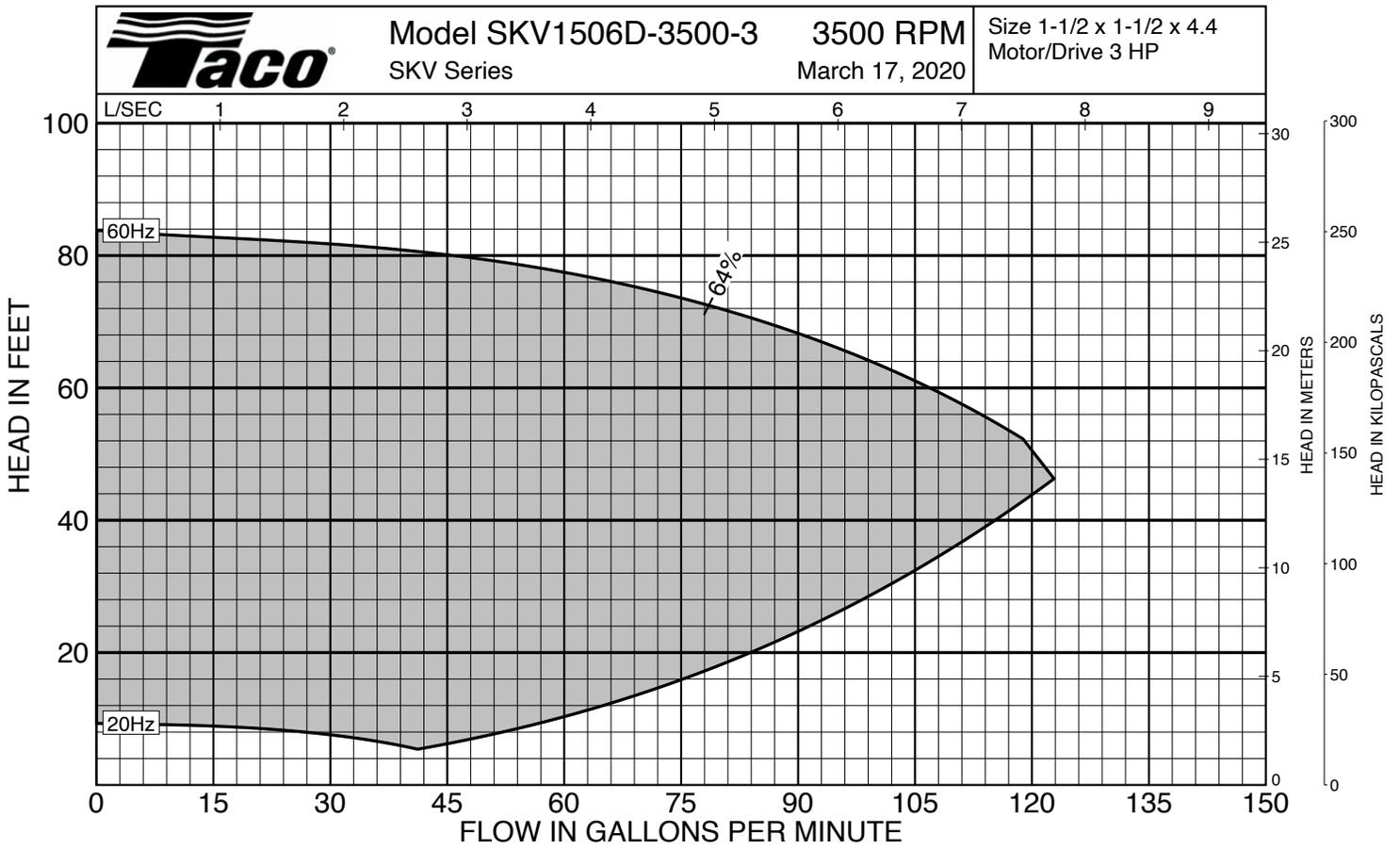
Curves based on Clear Water @ 60F with a Specific Gravity of 1.0
