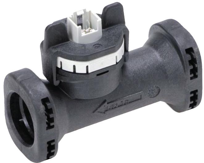
The flow sensor type 200 is based on the Kármán vortex trail. Vortex trail principle and is available in various options with and without temperature measurement. With no moving parts the flow sensor is not sensitive to debris, has marginal pressure loss and high accuracy.
