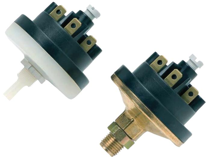
Type 620 and 625 pressure switches, with 13 pressure ranges, are suitable for liquids and gases. Body materials are available in plastic, brass and aluminium, with a choice of NBR, FPM, EPDM and silicone diaphragms.
