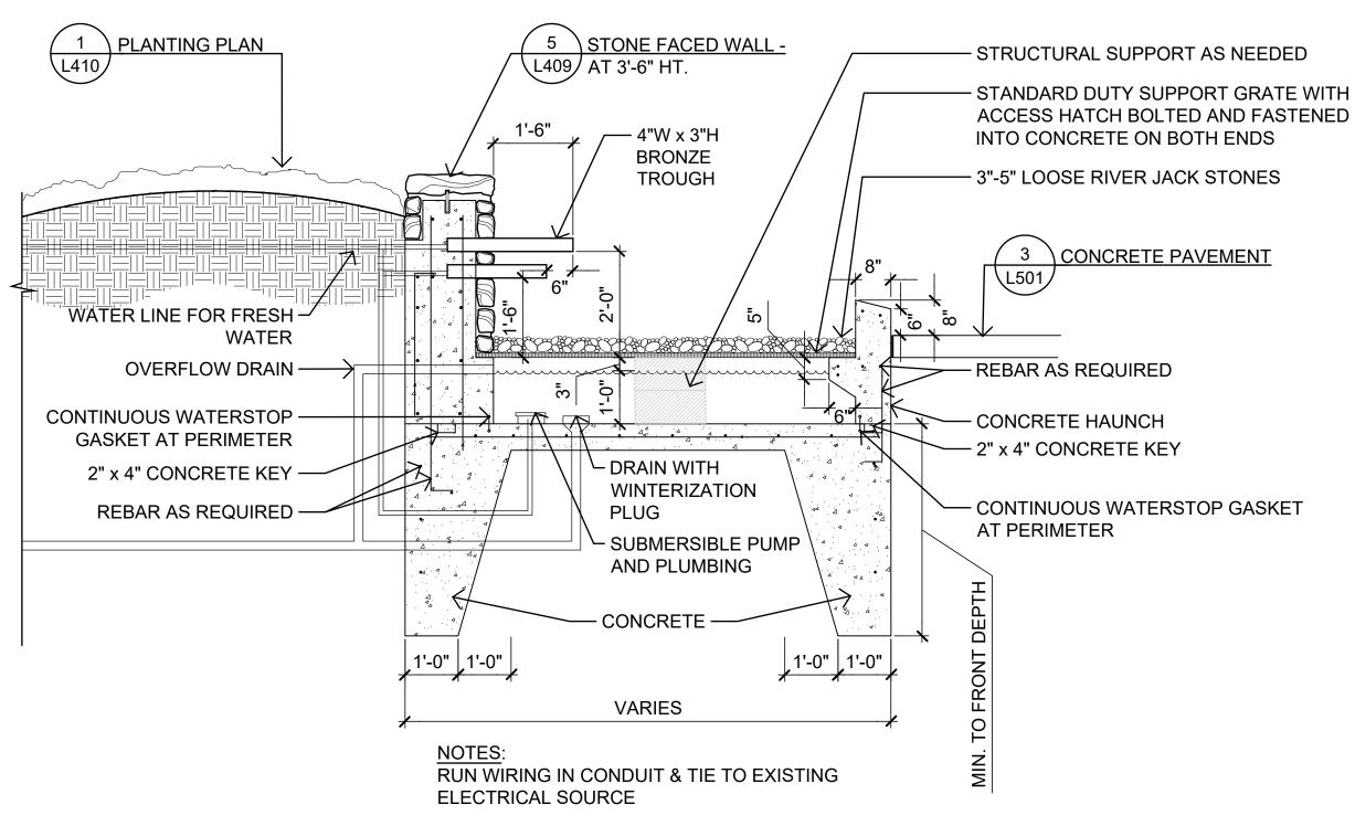
WATER FEATURE SCALE: 1/2" = 1'-0" 1. ALL BLOCKS SHALL HAVE HAND-TIGHT JOINTS, WITH A MAXIMUM GAP OF 3/8" - 1/2" BETWEEN EACH BLOCK. 2. ALL STONE BLOCKS SHALL BE CUT RADIALLY, WITH MAX 3/8" - 1/2" JOINT. LINEAR DIMENSION LINEAR DIMENSION
