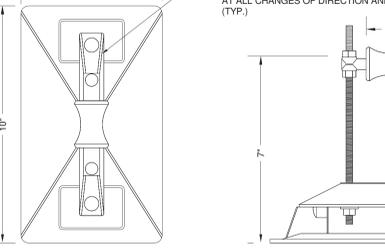
18 GAS PIPE ROOF SUPPORT DETAIL
