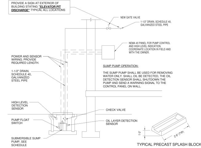
9 ELEVATOR SUMP PUMP PIPING DETAIL
