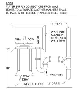
3 WASHING MACHINE RECESSED WALL BOX DETAIL (ELEVATION)
