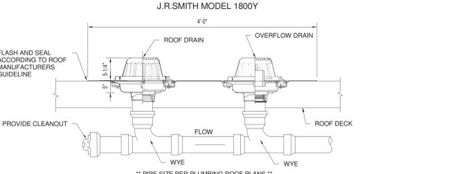
14 ROOF DRAIN AND OVERFLOW DRAIN COMBINATION PIPING DETAIL
