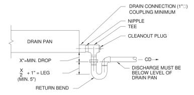
2 CONDENSATE DRAIN TRAP DETAIL
