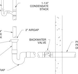
17 CONDENSATE DRAIN STAND PIPE DETAIL
