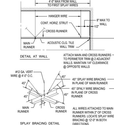
**A** A5.00 3/8" = 1'-0" **Typ. Seismic Bracing**
