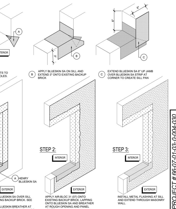
**12 Unit Ventilator/Window Flashing Detail**
