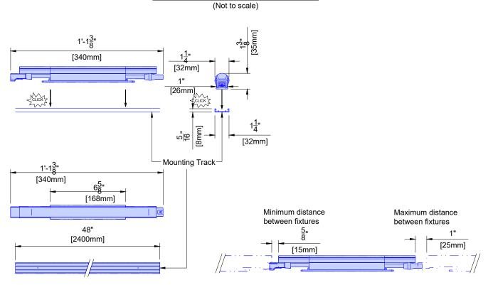
\*\*Recommended mounting clear plastic covers on a track for ease of service. Sufficient ventillation must be provided to closed coves to remove heat given off by LEDs.
