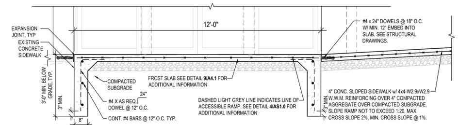
4 CONCRETE SLOPING SIDEWALK SECTION
