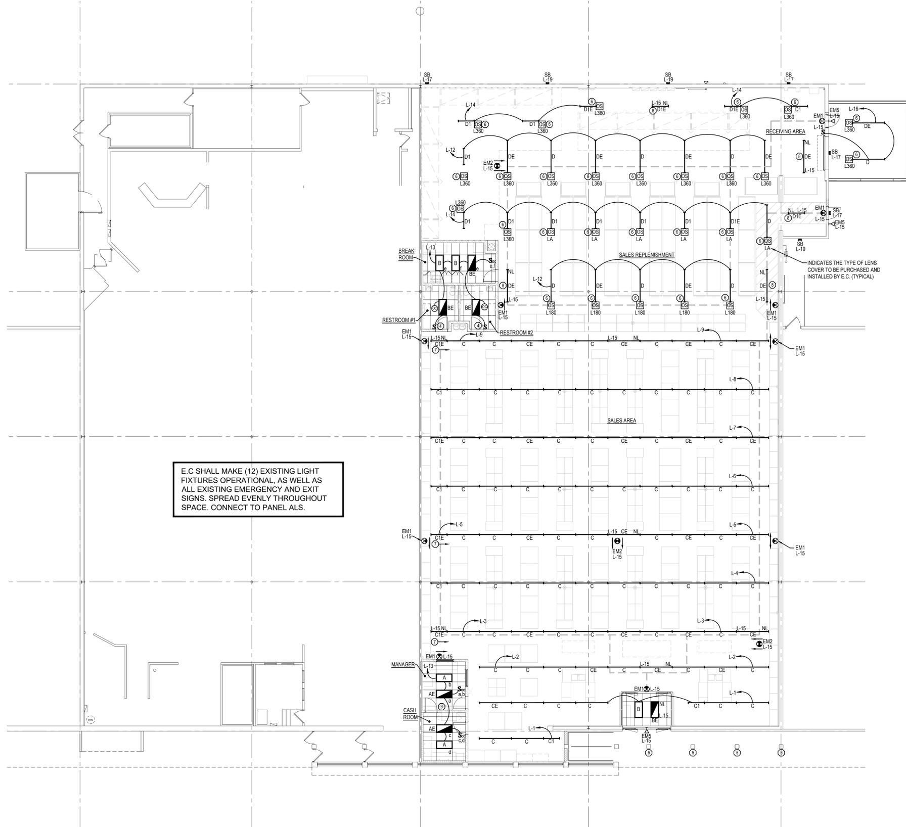
E.C SHALL MAKE (12) EXISTING LIGHT FIXTURES OPERATIONAL, AS WELL AS ALL EXISTING EMERGENCY AND EXIT SIGNS. SPREAD EVENLY THROUGHOUT SPACE. CONNECT TO PANEL ALS.
