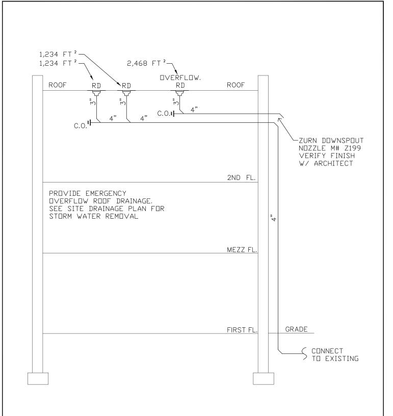
NOTE: PIPE SIZING BASED UPON 1/8"/FT SLOPE.
