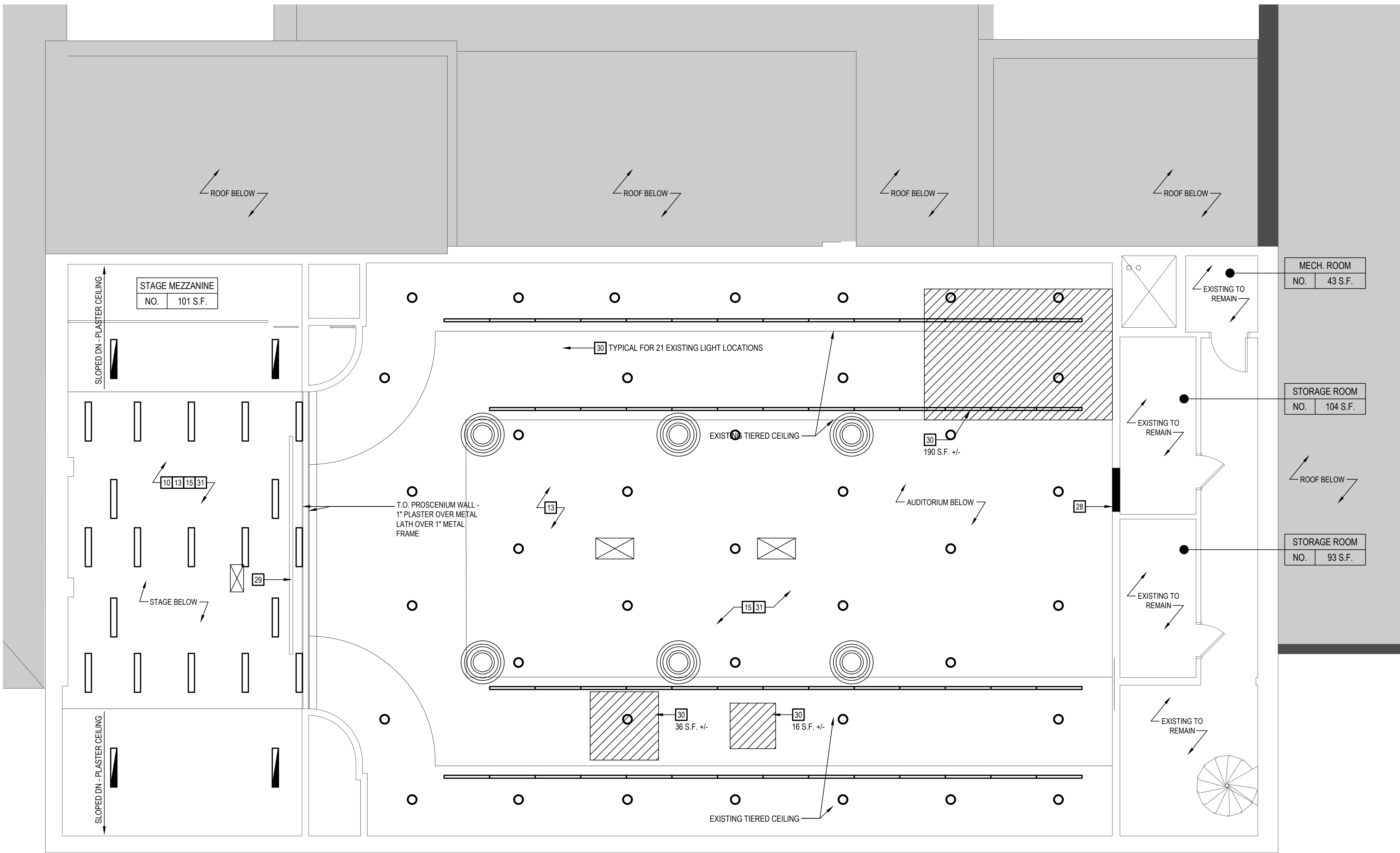
1 Auditorium Reflected Ceiling Plan SCALE: 3/16"=1'-0"
