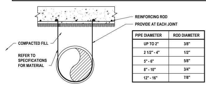
**Underground Piping Support Below Slab Detail**
