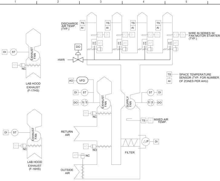
**AIR HANDLING UNIT - MULTI-ZONE, HOT WATER (WITH LAB HOOD EXHAUST) - SEQUENCE OF OPERATIONS:**
