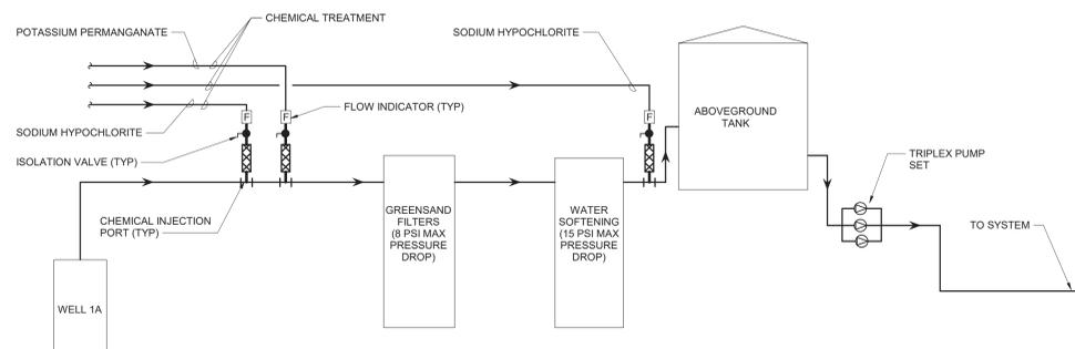
4 Water Treatment Hydraulic Schematic
