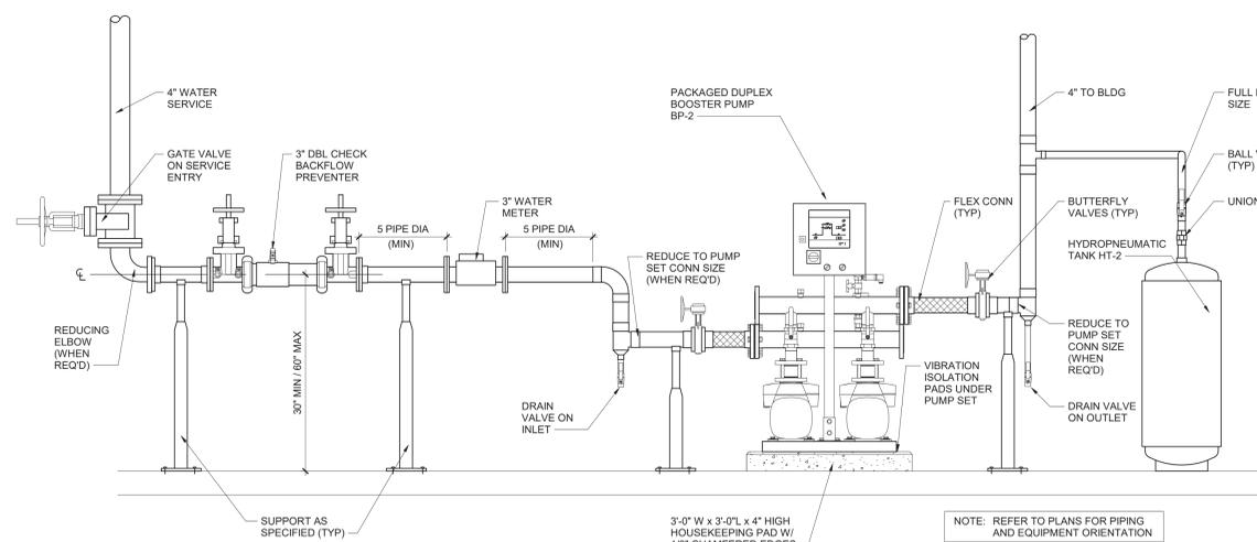
**7 Duplex Booster Pump System Schematic**
