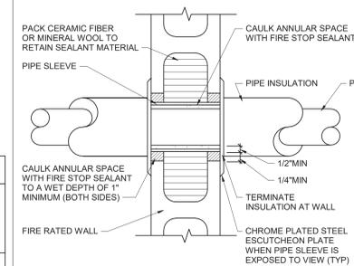
**3 Fire Rated CMU Wall Pipe Sleeve Detail**
