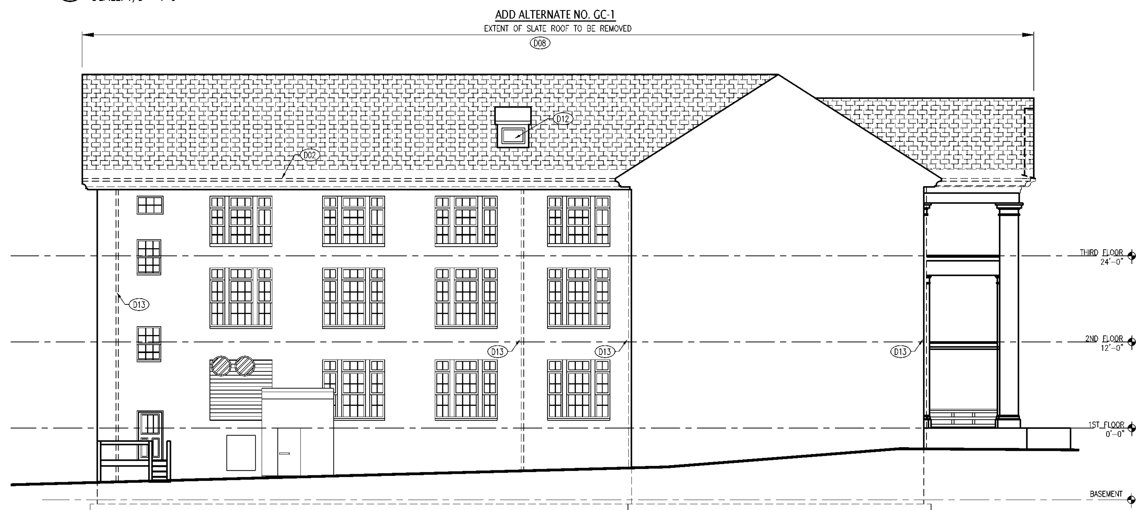
3 SOUTH ELEVATION OF CENTRAL WING: REMOVALS SCALE: 1/8" = 1'-0"
