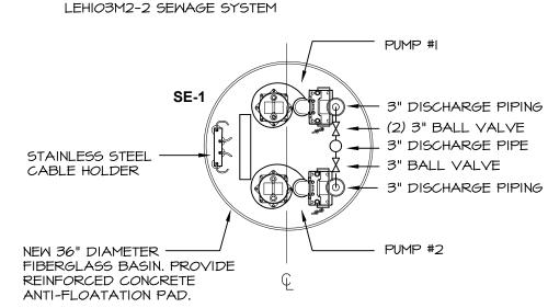
DUPLEX SEWAGE EJECTOR (SE-I) PLAN DETAIL
