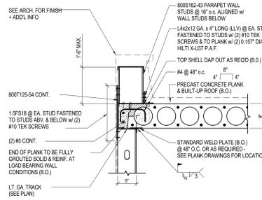
10 LOW PARAPET WALL SECTION
