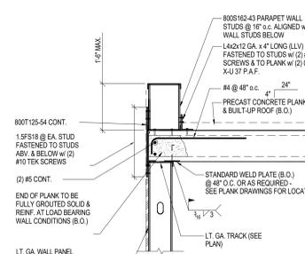
9 LOW PARAPET WALL SECTION
