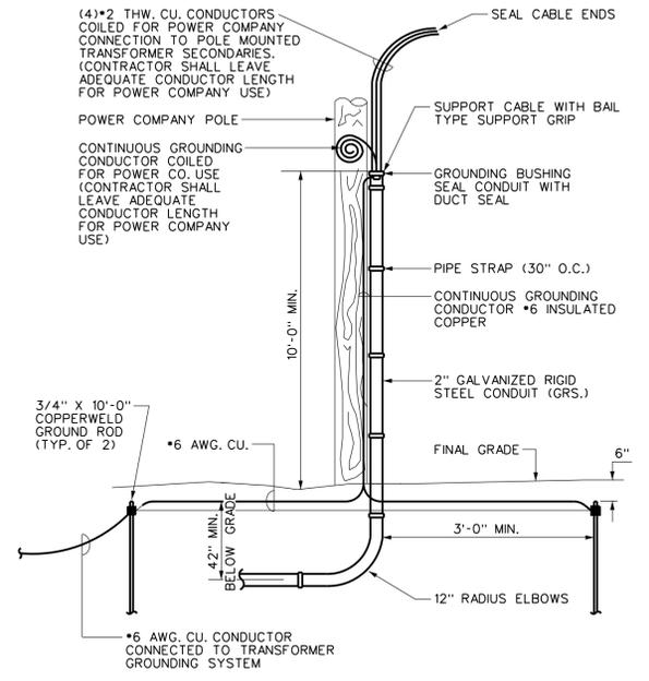
**3 UTILITY POLE CONDUIT RISER DETAIL**
