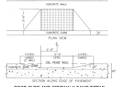
DROP CURB AND SIDEWALK RAMP DETAIL
