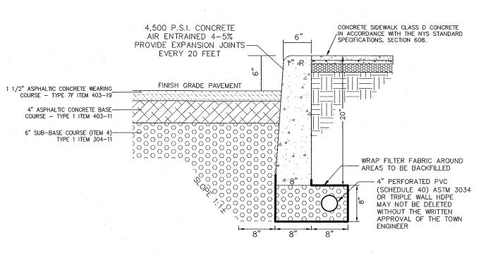
ASPHALTIC CONCRETE PAVEMENT & CONCRETE CURB DETAIL FOR TRAVELLED WAY
