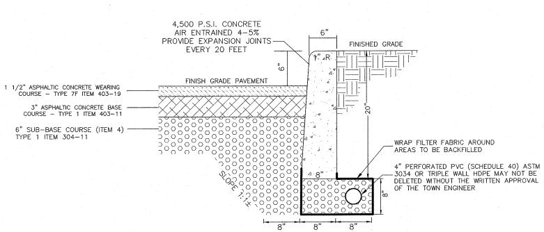
ASPHALTIC CONCRETE PAVEMENT & CONCRETE CURB DETAIL FOR PARKING AREAS
