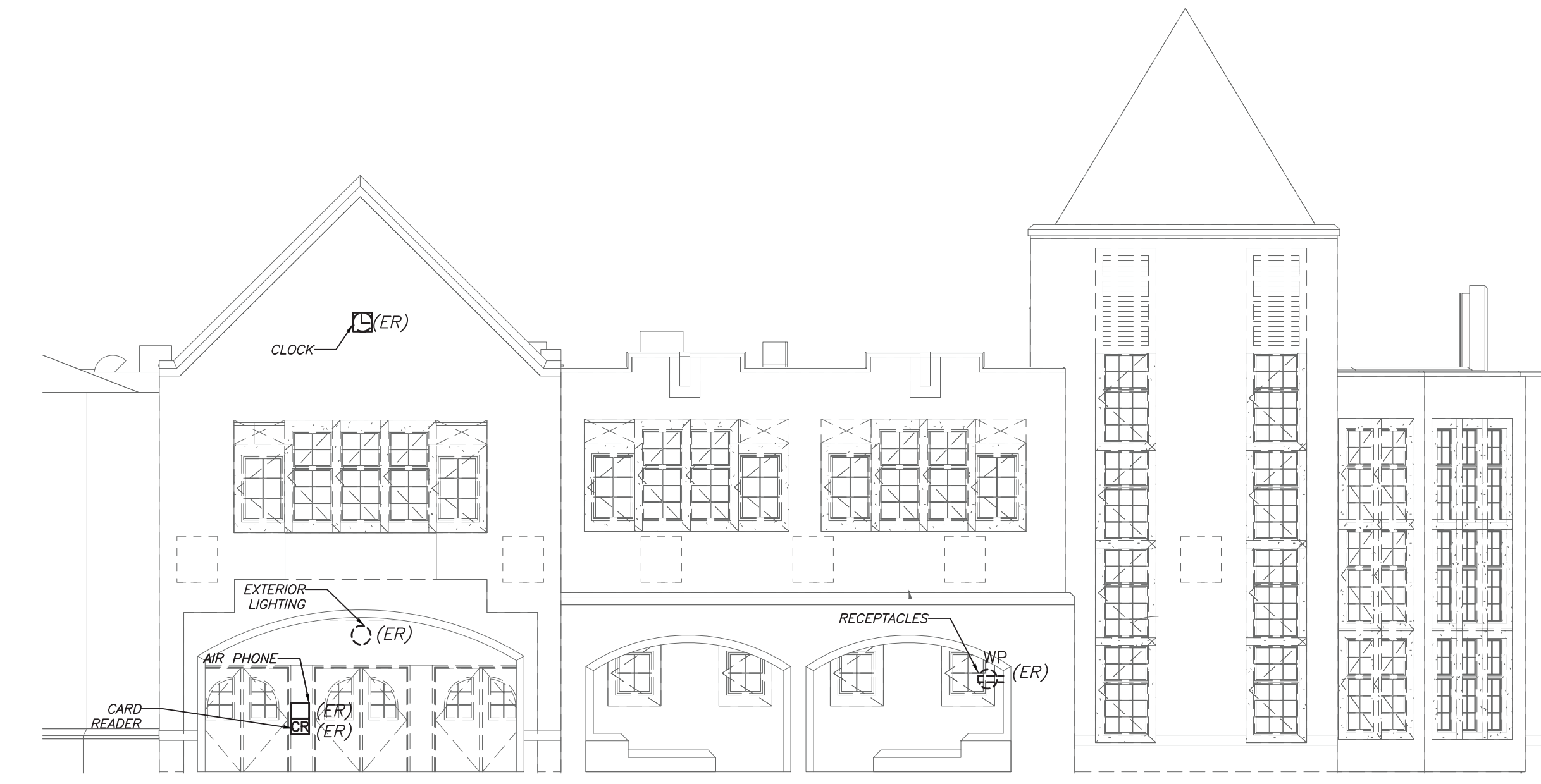
EXTERIOR POWER PLAN (NEW WORK) (PROJECT 4) 1 E2-312
