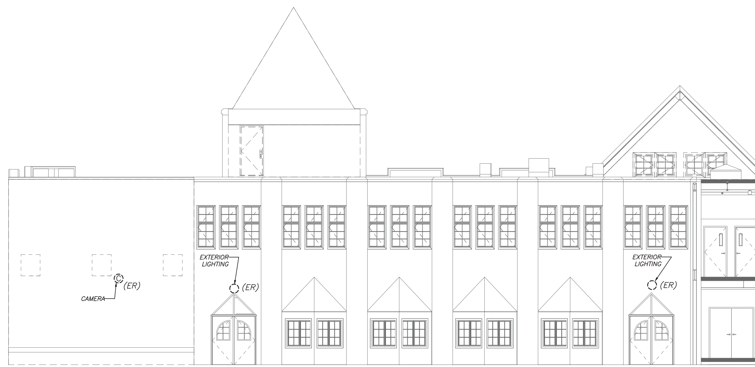
EXTERIOR POWER PLAN (NEW WORK) (PROJECT 4) 4 E2-312
