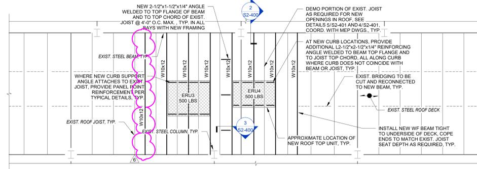
**5 PARTIAL ROOF FRAMING PLAN**
