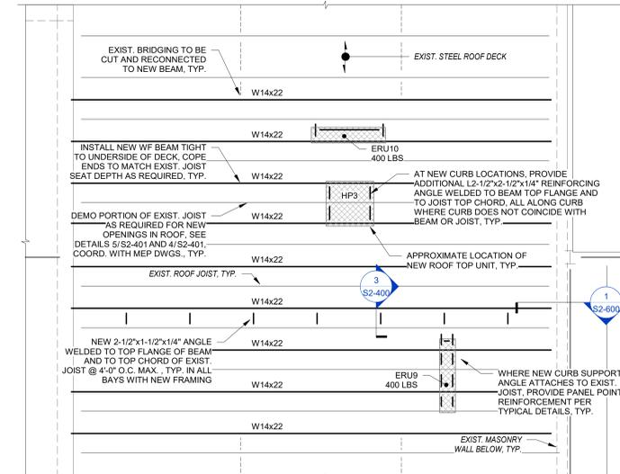
**3 PARTIAL ROOF FRAMING PLAN**
