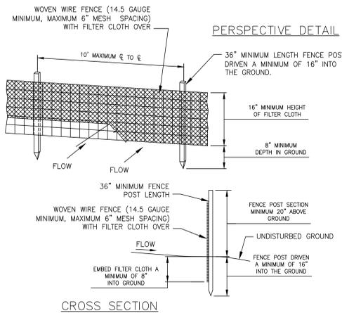
CONSTRUCTION NOTES FOR FABRICATED SILT FENCE
