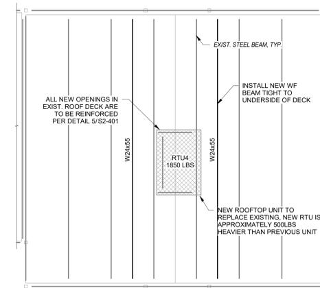
**6 PARTIAL ROOF FRAMING PLAN**
