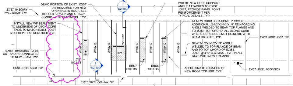
**2 PARTIAL ROOF FRAMING PLAN**
