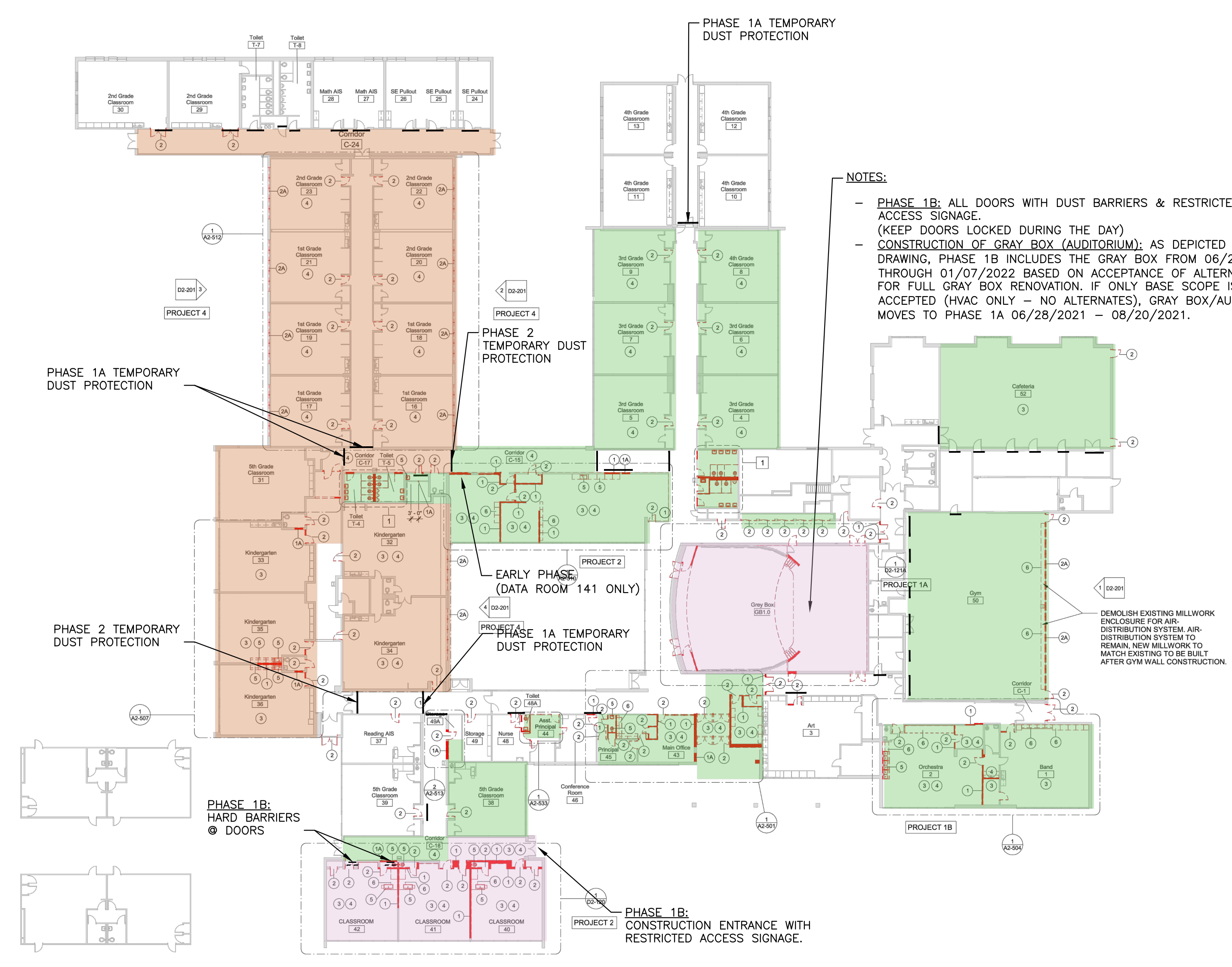
CONSTRUCTION IMPLEMENTATION PLAN - FIRST FLOOR
