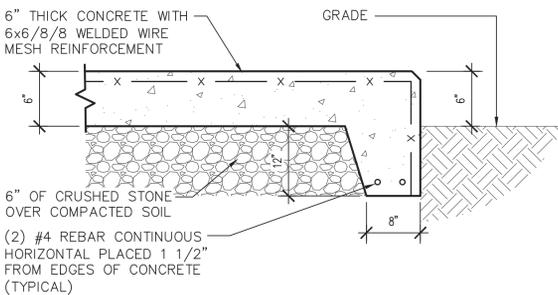
**2 CONCRETE EQUIPMENT SUPPORT PAD DETAIL**
