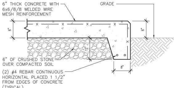
**2 CONCRETE EQUIPMENT SUPPORT PAD DETAIL**
