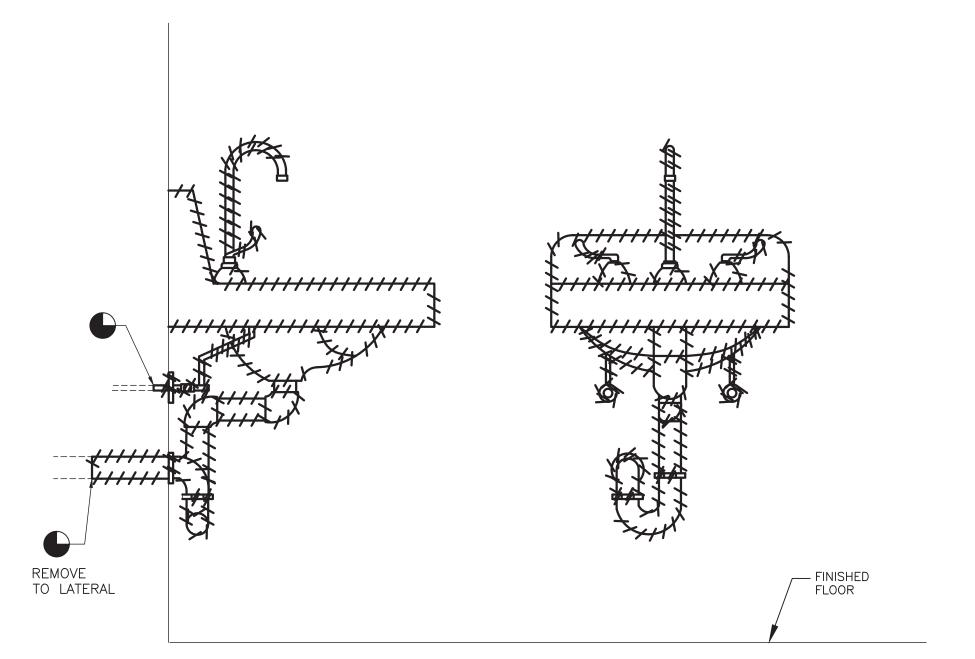
1. REMOVE LAVATORIES, CARRIERS AND ASSOCIATED. REMOVE SANITARY, HOT & COLD WATER SUPPLIES TO WALL/LATERAL. (WATER CLOSETS AND URINALS SIMILAR)
