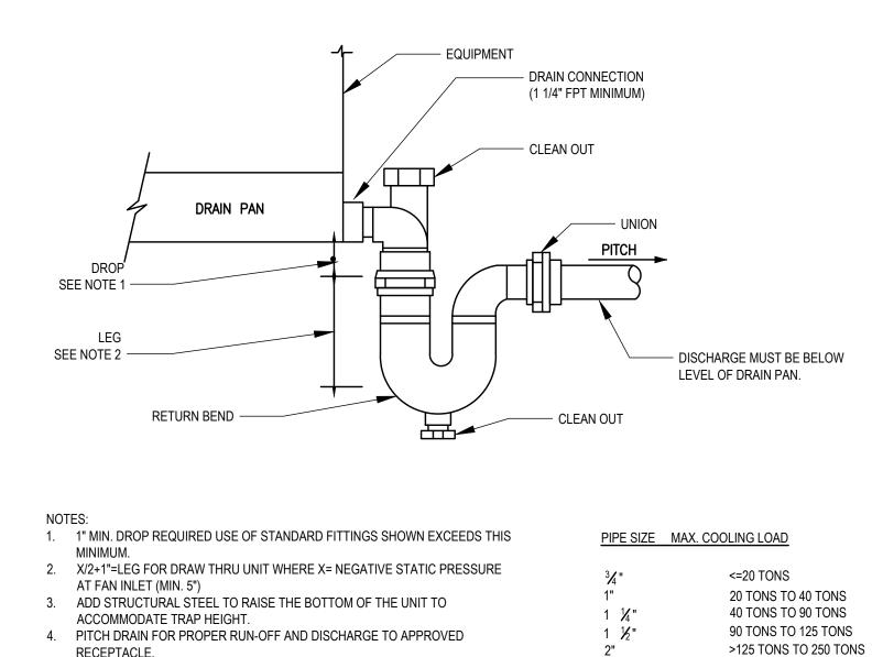
RECEPTACLE. 5. SUPPORT DRAIN LINES TO PREVENT SAG AND CONDENSATE OVERFLOW.
