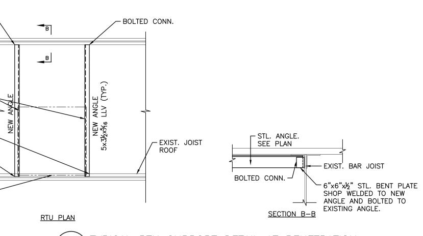
2 TYPICAL RTU SUPPORT DETAIL AT PENETRATION SD-100 SCALE: N.T.S.
