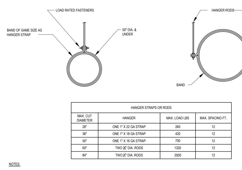
1. TABULATED DATA FROM SMACNA ALLOWS FOR DUCT REINFORCING AND INSULATION, BUT NO EXTERNAL LOAD. 2. INSULATION AROUND HANGER.
