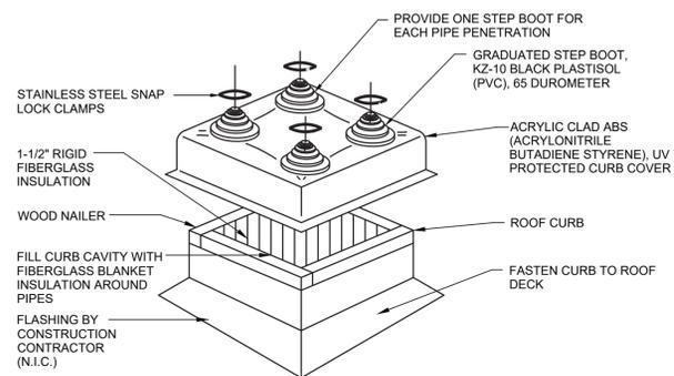
**8 MECHANICAL REFRIG. PENETRATION DETAIL**
