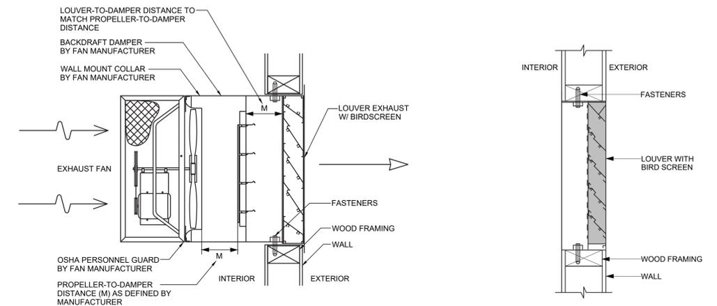
**6 PROPELLER FAN DETAIL**
