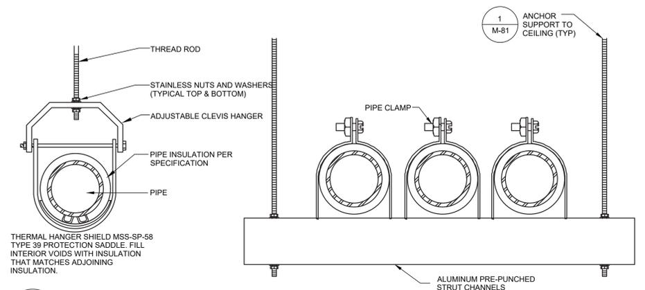
**3 MECHANICAL PIPE HANGER DETAIL**
