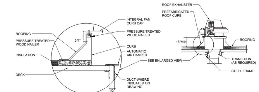
**9 MECHANICAL ROOF FAN DETAIL**
