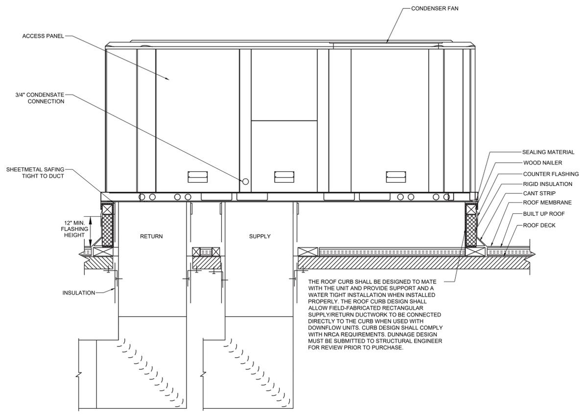
**2 ROOF TOP UNIT (RTU) DETAIL**
