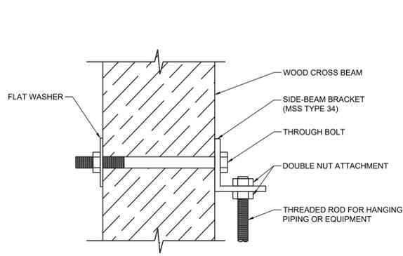
**1 MECHANICAL ANCHORING DETAIL**
