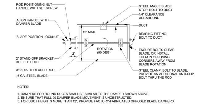
**3 MECHANICAL VOLUME DAMPER DETAIL**
