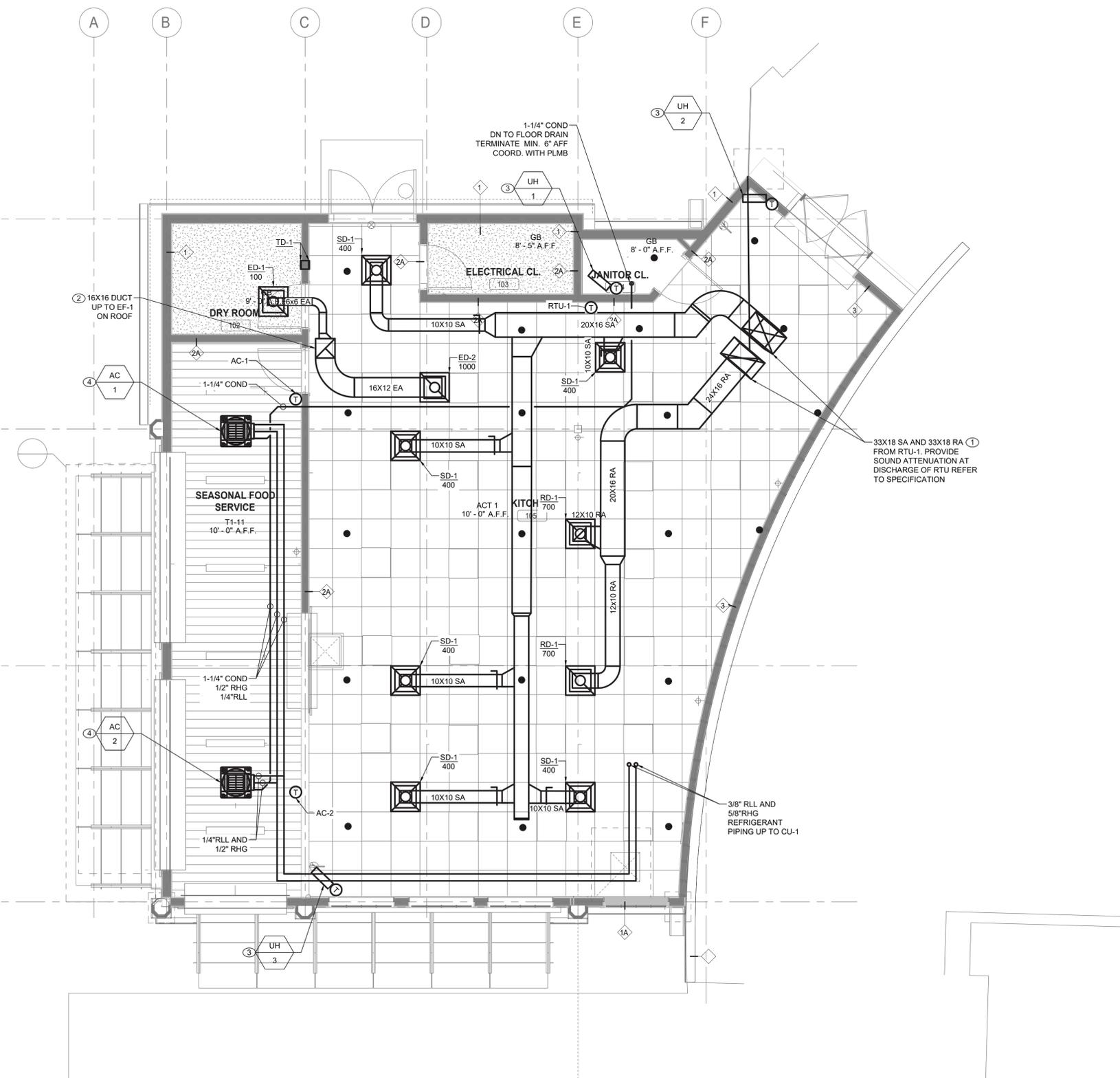
**1 MECHANICAL FIRST FLOOR CONSTRUCTION PLAN**
