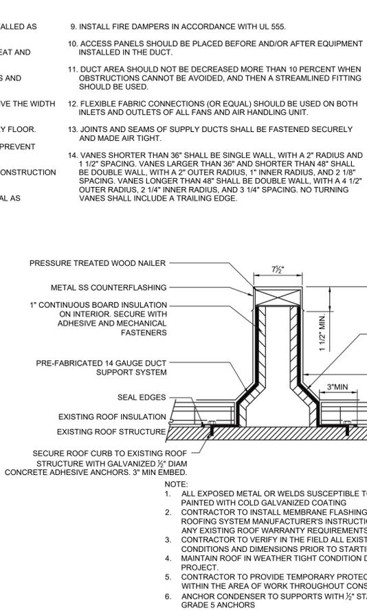
**4 MECHANICAL EQUIP RAILS DETAIL**
