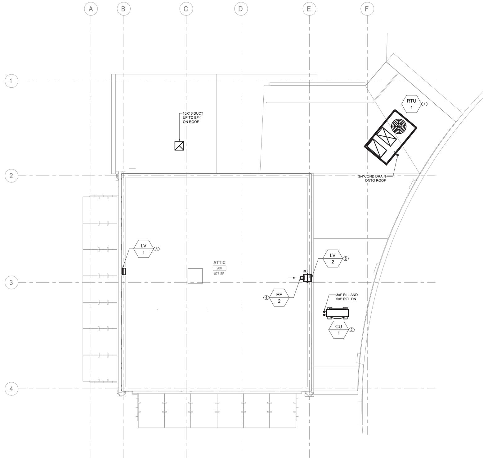
**1 MECHANICAL ATTIC FLOOR CONSTRUCTION PLAN**
