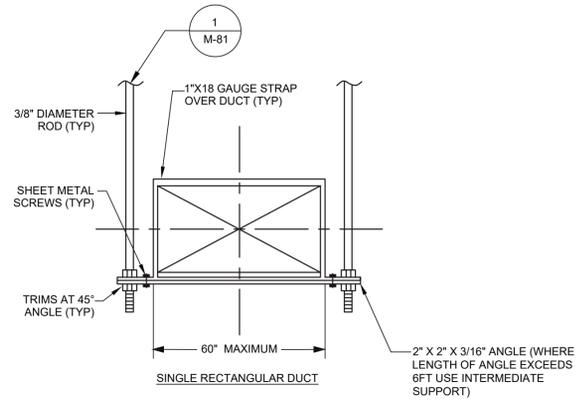
**2 MECHANICAL DUCT HANGER DETAIL**
