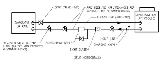
**5 DX COIL PIPING DIAGRAM**
