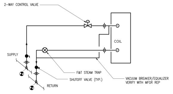
**4 STEAM COIL PIPING AT UV DETAIL**
