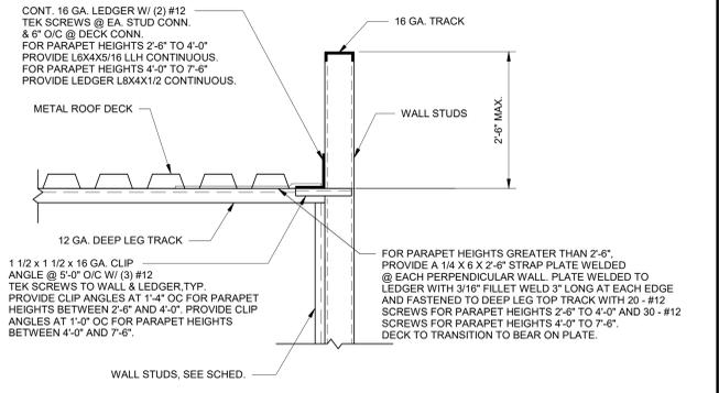
**4 TYPICAL DETAIL @ PERIMETER ROOF EAVE W/ PARAPET**
