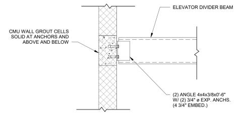
**11 ELEVATOR HOIST BEAM ATTACHMENT DETAIL TO CMU WALL**
