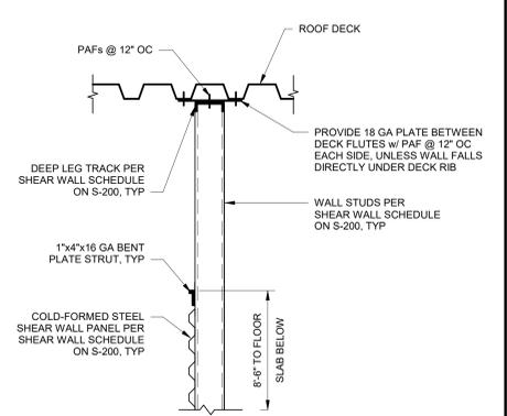
**9 TYPICAL SHEAR WALL DETAIL AT ROOF**
