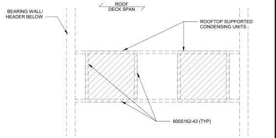
**13 TYPICAL ROOF TOP CONDENSING UNIT FRAMING PLAN**
