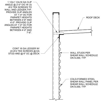
**6 TYPICAL EXT SHEAR WALL BEARING DETAIL AT ROOF**
