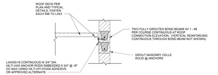
**10 ROOF LEDGER TO MASONRY WALL WHERE WALL EXTENDS ABOVE ROOF**
