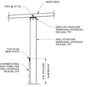
**8 TYPICAL SHEAR WALL BEARING DETAIL AT ROOF**
