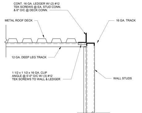
**3 TYPICAL DETAIL @ PERIMETER ROOF EAVE**
