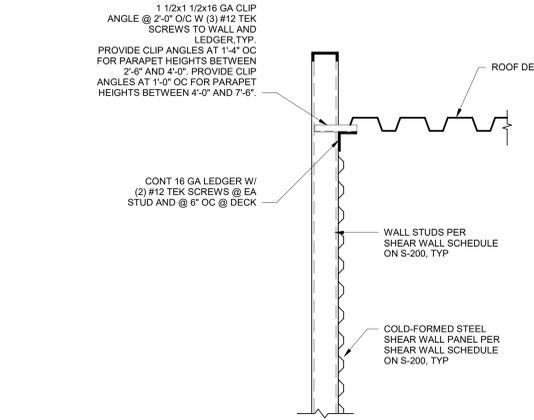
**7 TYPICAL EXT SHEAR WALL DETAIL AT ROOF**
