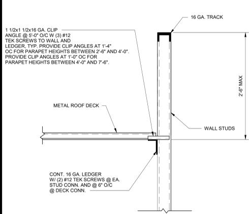
**5 TYPICAL DETAIL @ PERIMETER AT RAKE**
