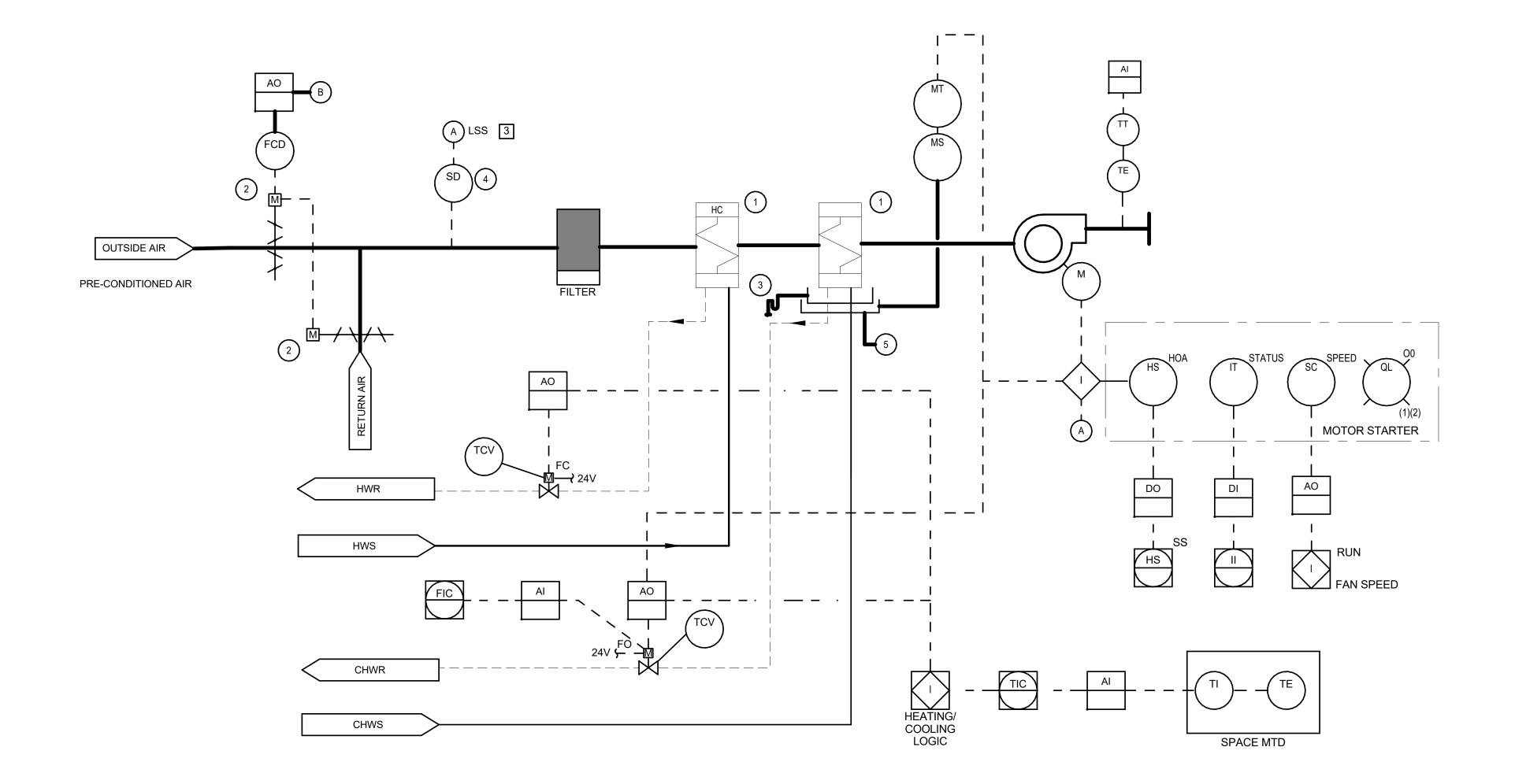
1 TYPICAL 4-PIPE HORIZONTAL FAN COIL UNIT W/ MIXING BOX P&ID
