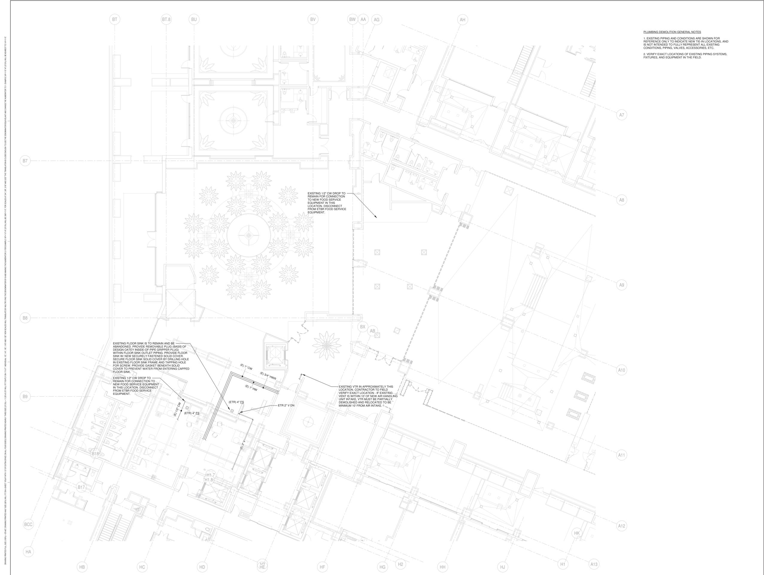
EXISTING FLOOR SINK IS TO REMAIN AND BE ABANDONED. PROVIDE REMOVABLE PLUG (BASIS OF DESIGN DATE) INSIDE-OF-PIPE GRIPPER PLUG) WITHIN FLOOR SINK OUTLET PIPING. PROVIDE FLOOR SINK W/ NEW SECURELY FASTENED SOLID COVER. SECURE FLOOR SINK SOLID COVER BY DRILLING HOLE IN EXISTING FLOOR SINK FRAME AND TAPPING HOLE FOR SCREW. PROVIDE GASKET BENEATH SOLID COVER TO PREVENT WATER FROM ENTERING CAPPED FLOOR SINK.
