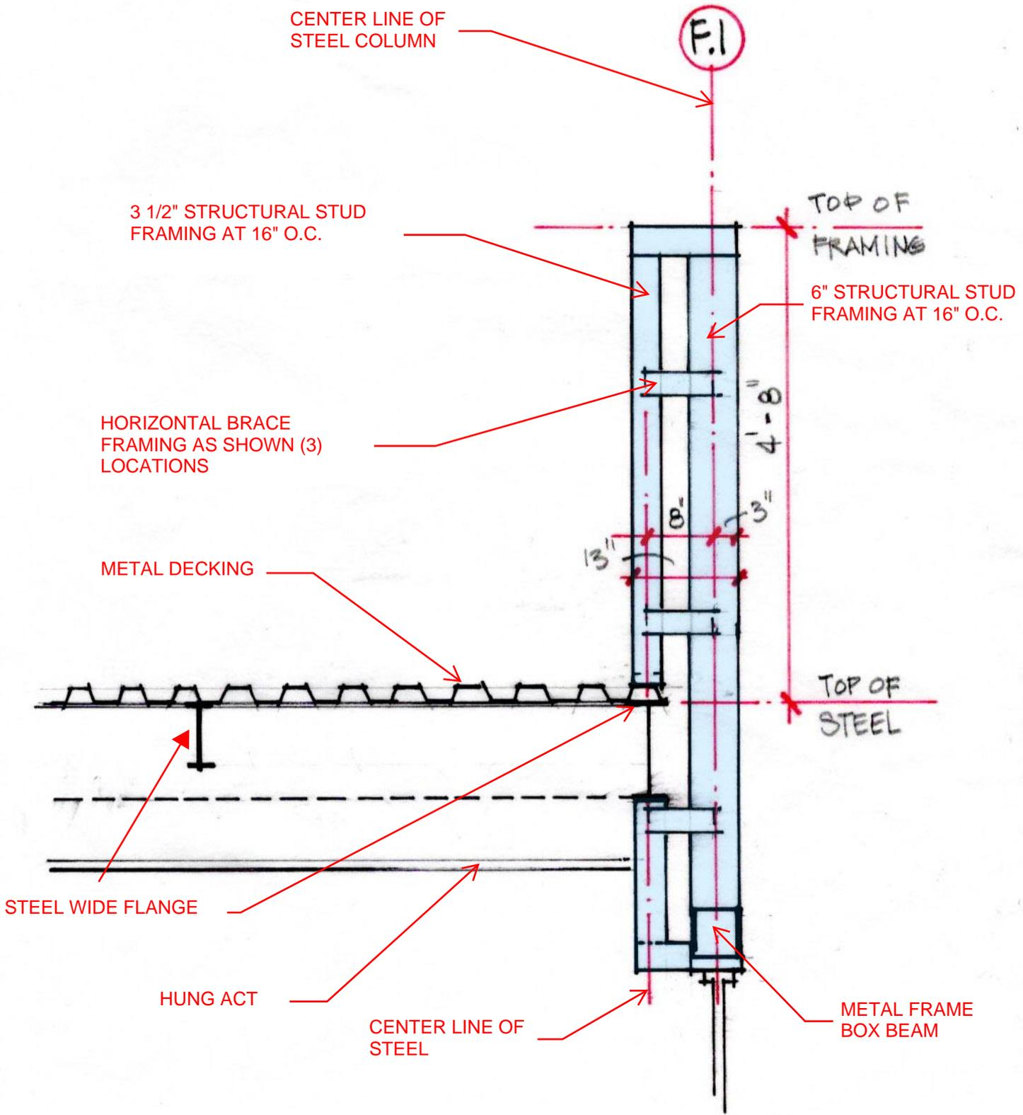
STRUCTURAL STEEL AND METAL COLD-FORMED FRAMING SHOWN ONLY. FOR MATERIALS SEE ARCHITECTURAL DETAILS DETAILS. SK-3 APPLIES TO ALL SLOPED GLAZING CONDITIONS
