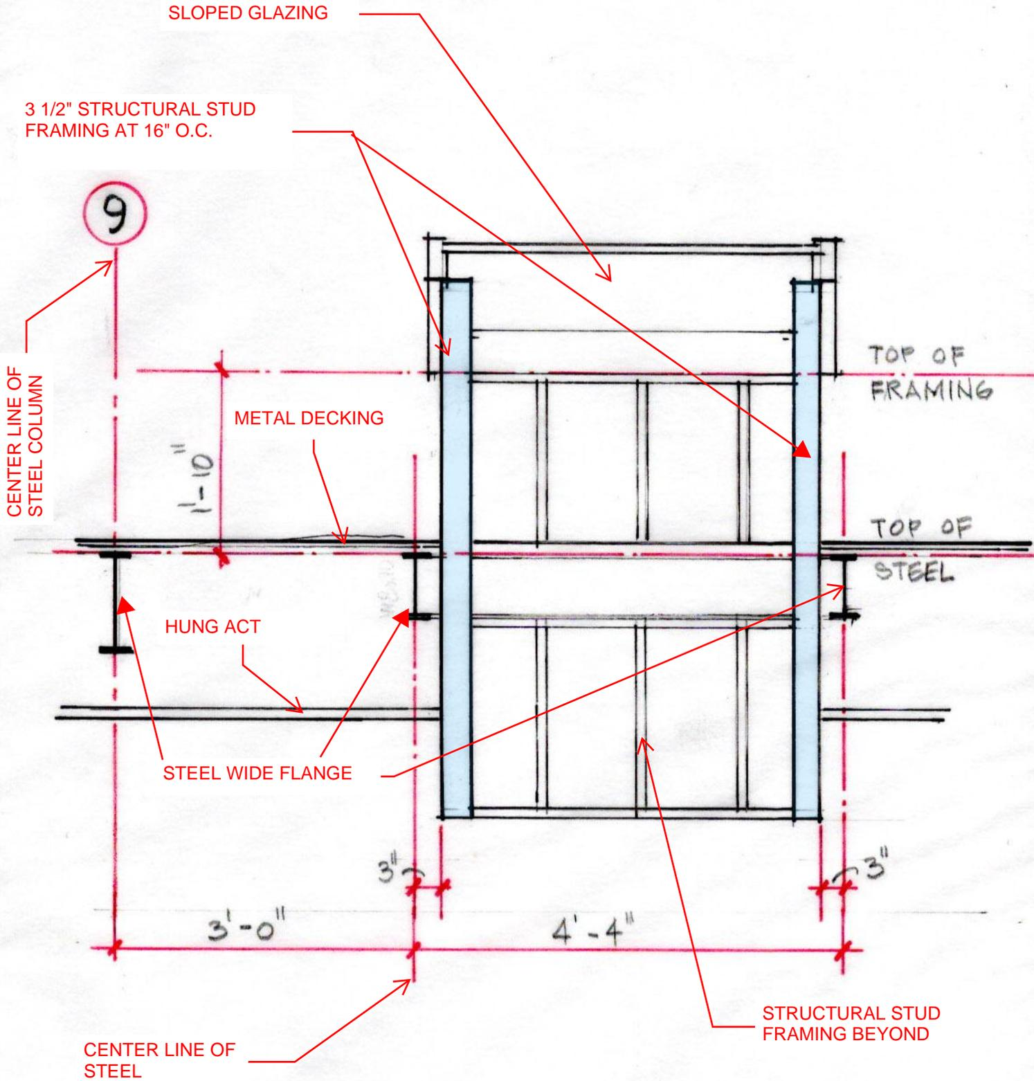
STRUCTURAL STEEL AND METAL COLD-FORMED
