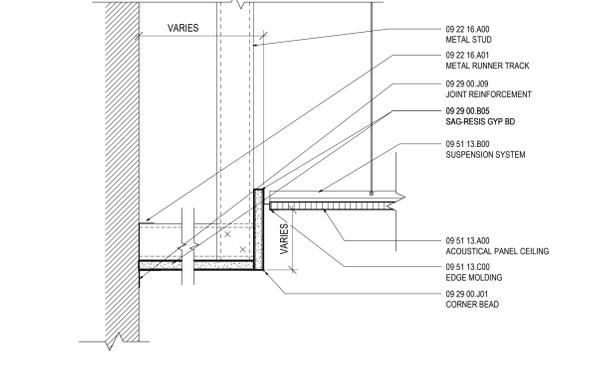
**03 SECTION DTL - CLG SOFFIT / FASCIA**
