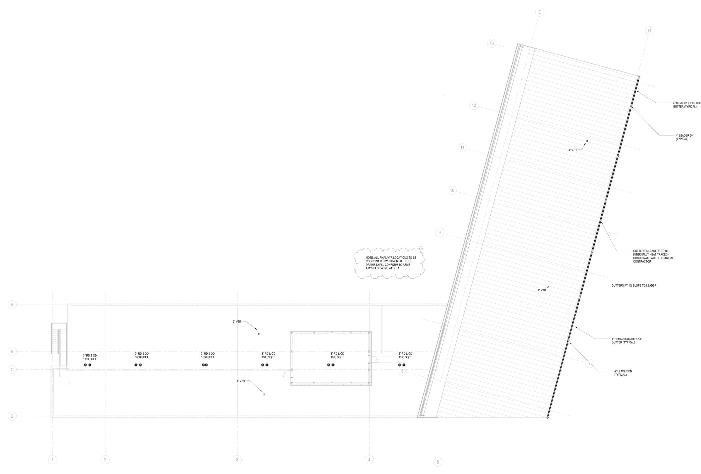
NOTE: ALL FINAL VTR LOCATIONS TO BE COORDINATED WITH RGN. ALL ROOF DRAINS SHALL CONFORM TO ASME A112.6.4 OR ASME A112.3.1
