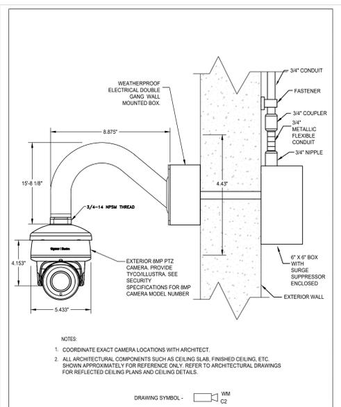
**OUTDOOR IP FIXED CAMERA MOUNTED TO THE WALL** 04
