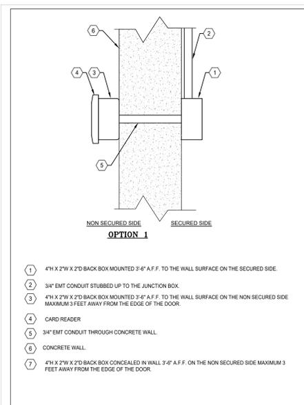
**TYPICAL CARD READER CONCRETE WALL INSTALLATION DETAIL** 01
