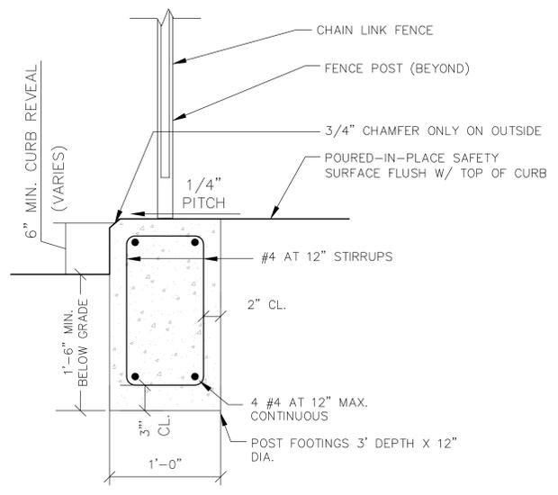
**3 CAST-IN-PLACE CONTINUOUS CONCRETE FENCE CURB**
