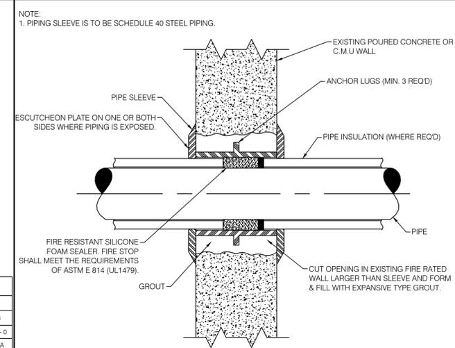
**1** PIPE PENETRATION THROUGH FIRE RATED WALL
